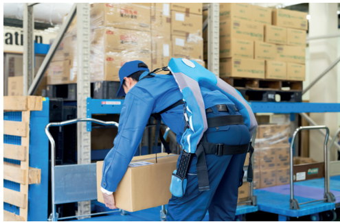
Left: Application example for exoskeletons as assistance systems for physical activities in logistics, Photo: © metamorworks/adobe stock.com | Above: Sensor-supported process recording and tool-based requirements analysis, Photo: © Mediaparts/adobe stock.com
