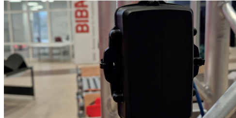
Left: Mobile crane in use on a construction site, Photo: © Roman_23 203/stock.adobe.com | Above: Sensor module for identifying and monitoring the condition of crane components in the test environment, Photo: BIBA GmbH
